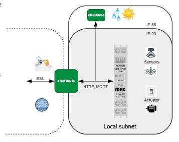
All software interfaces are based on open protocols. Thus, all devices can be operated directly in your network environment without registration, app or cloud connection. This offers the highest possible protection for your data.
